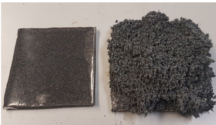
Figure 1 - A steel plate coated with a 0.3mm thick GrafGuard expandable graphite centered epoxy coating before and after exposing to a flame. The expanded char measured nearly 100mm thick.
